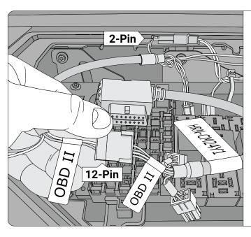
Note: For Volvo vehicle models from 2004 to 2007 where the 2-pin gray J1939 connector is not available — Plug the 2-pin black connector of the HRN-CE10A2 (green and brown wires) into the mating 2-pin black connector in the top passenger corner of the fuse box. Next, connect the 12-pin black Molex connector on the HRN-CE10A2 to the corresponding connector on the HRN-CM24Y1. They are both labeled OBDII.
