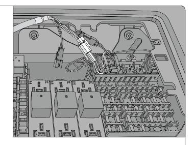
**Step 4:** Remove the terminating resistor and then plug it into the mating end of the HRN-CE10A2. Connect the HRN-CE10A2 to where the terminating resistor was removed.
