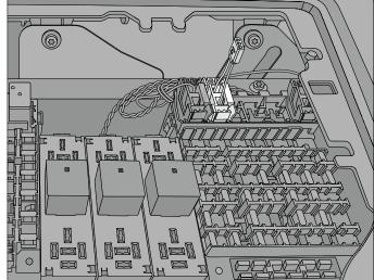
**Step 2:** Connect the 2-pin white connector from the kit into any spare constant power slot. Test for power with a multimeter to verify.
