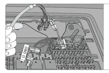
**Step 3:** Connect the other end of the connector to the 2-pin black connector on HRN-CE10A2.
