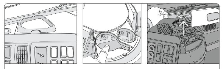
Step 1: Remove the two T-25 screws holding the fuse box cover in place, then pull gently upward to remove the cover.
